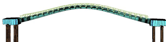
Fig. 10. First Mode 2.8 Hz (Bending)
